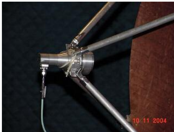
Fig 6.1 : Ku band Feed with Piezo Coated Teflon spars
