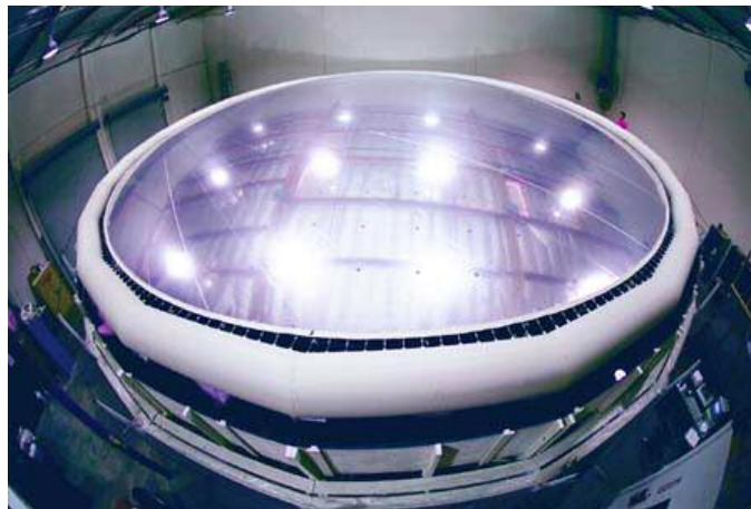
Fig 2.6: A typical NASA's Inflatable Antenna Experiment reflector during ground tests
